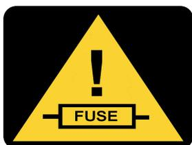
**INSTALLEZ LE FUSIBLE DE PROTECTION FOURNI SUR LE CÔTÉ DE LA BATTERIE AU DÉBUT DE LA LIGNE D'ALIMENTATION.**
