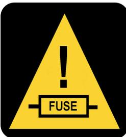
TOUJOURS INSTALLER LE FUSIBLE DE PROTECTION AU DÉBUT DE LA LIGNE D'ALIMENTATION ET RÉALISER TOUTES LES CONNEXIONS ÉLECTRIQUES CONFORMÉMENT AUX INSTRUCTIONS POUR PERMETTRE LE FONCTIONNEMENT APPROPRIÉ DES DISPOSITIFS DE SÉCURITÉ.
