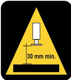
LA DISTANCE D'INSTALLATION MINIMUM ENTRE LE SOL ET LA BASE DU VÉRIN DOIT ÊTRE COMPRISE ENTRE 30 ET 40 MM MIN, LORSQUE LES VÉRINS SONT EN POSITION VERTICALE.
