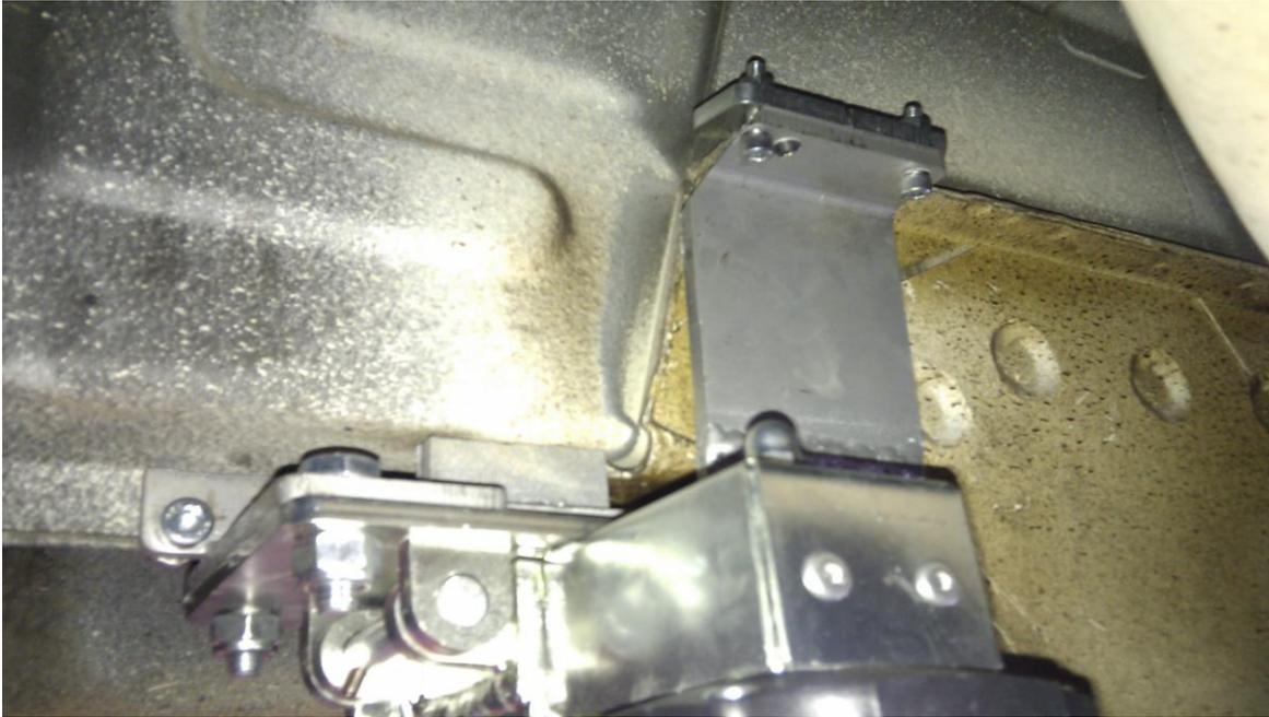
Put the adapter most front possible, if necessary remove any sealing material for a perfect adherence, use a bottle jack to stop the bracket in the correct position and make the 8mm side hole then fix with the bolt.
