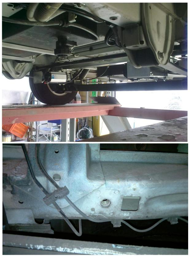
The rear adapter must be placed before the rear axle
