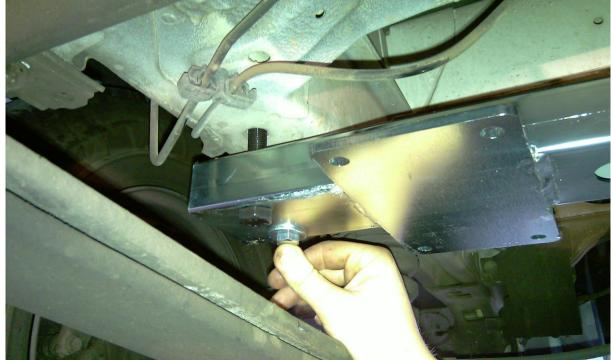
Step 2: Insert and position the sealing plate then fix with the bolts.
