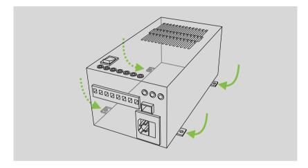
THE IDEAL MOUNTING POSITION IS SMOOTH, WELL VENTILATED AND NOT SUBJECT TO OVERHEATING; AVOID SURFACES COVERED WITH FABRIC OR CARPET. INSTALL THE DEVICE AS CLOSE AS POSSIBLE TO THE SERVICE BATTERIES.
